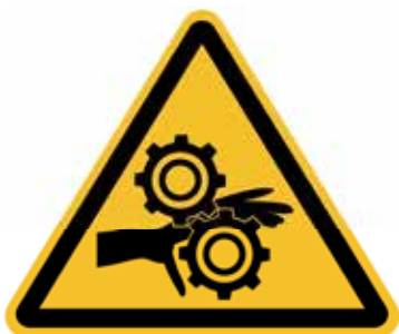
Do not place your hands in the drive system! There is danger of bodily harm!
